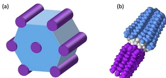
**Fig. 5** (a) Schematic representation of Col<sub>h</sub> packing of compounds 2–4 showing nano-segregated hydrophilic (purple) and hydrophobic domains (blue); model of 2 showing PEG chains (purple), CD (white) and hydrophobic chains (blue).
