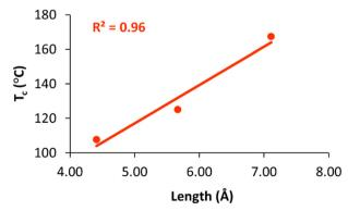
Fig. 6 Plots of clearing temperature  $(T_c)$  versus dipole moment (top) and length of the terminal group (bottom).
