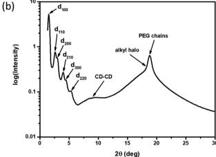
Fig. 4 X-Ray diffractograms of 2 at (a) 95 °C (Col<sub>h</sub>) and (b) room temperature (Col<sub>h</sub>\*).
