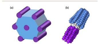
Fig. 5 (a) Schematic representation of Col<sub>h</sub> packing of compounds 2-4 showing nano-segregated hydrophilic (purple) and hydrophobic domains (blue); model of 2 showing PEG chains (purple), CD (white) and hydrophobic chains (blue).
