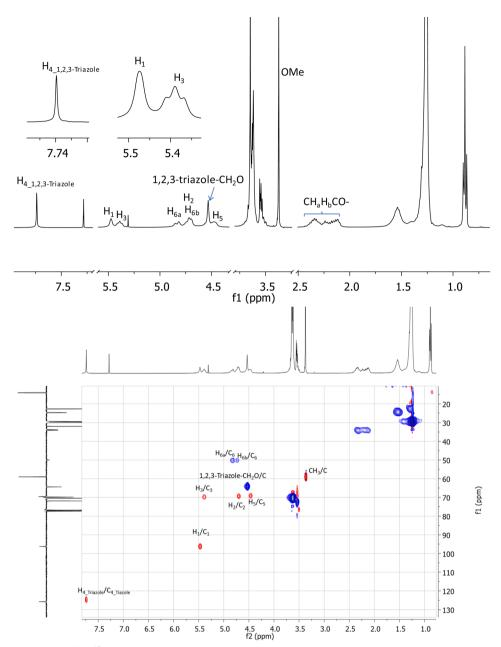
Fig. 2 <sup>1</sup>H NMR spectrum (top) and <sup>1</sup>H-<sup>13</sup>C gHSQC spectrum of synthesized compound **2** (CDCl<sub>3</sub>, 400 MHz).
