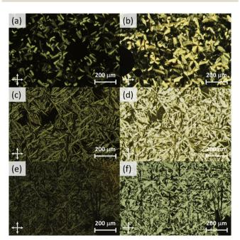
Fig. 3 Cross-polarized optical micrographs of 2 at (a) 99 °C (Col<sub>h</sub>) and (b) 39 °C (Col<sub>h</sub>\*), **3** at (c) 121 °C (Col<sub>h</sub>) and (d) 38 °C (Col<sub>h</sub>\*), and **4** at (e) 158 °C (Col<sub>h</sub>) and (f) 41 °C (Col<sub>h</sub>\*).
