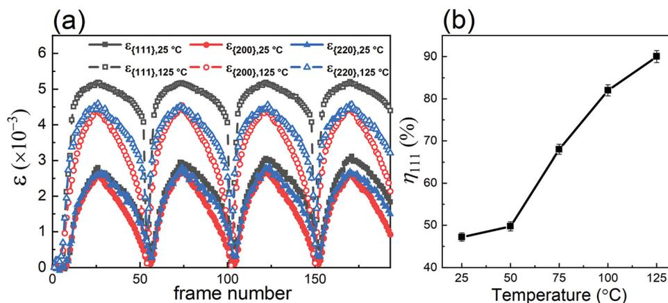
Fig. 8 (a) Influence of the applied electric field on effective lattice strains  $\varepsilon_{33}$  of Nb-doped 0.7BF–0.3BT ceramics for  $\{111\}_{\text{pc}}$ ,  $\{200\}_{\text{pc}}$  and  $\{220\}_{\text{pc}}$  at 25 and 125 °C. (b) Evaluated domain switching fraction,  $\eta$ , of (111) reflections, measured at various temperatures for the maximum field level.
