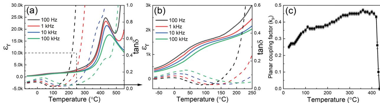
Fig. 4 (a) Temperature dependence of relative permittivity ( $\epsilon_r$ ) and loss ( $\tan \delta$ ) for  $0.7\text{BiFeO}_3-0.3\text{Ba}(\text{Ti}_{0.995}\text{Nb}_{0.005})\text{O}_3$  ceramics and (b) selected region illustrating variations in  $\epsilon_r$  and  $\tan \delta$  over the temperature range from  $-60$  to  $250$  °C (c) temperature-dependent planar coupling factor ( $k_p$ ).
