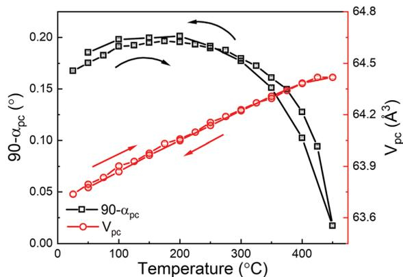
Fig. 2 Temperature dependence of rhombohedral lattice distortion and pseudo-cubic cell volume of  $0.7\text{BiFeO}_3-0.3\text{Ba}(\text{Ti}_{0.995}\text{Nb}_{0.005})\text{O}_3$  ceramics.
