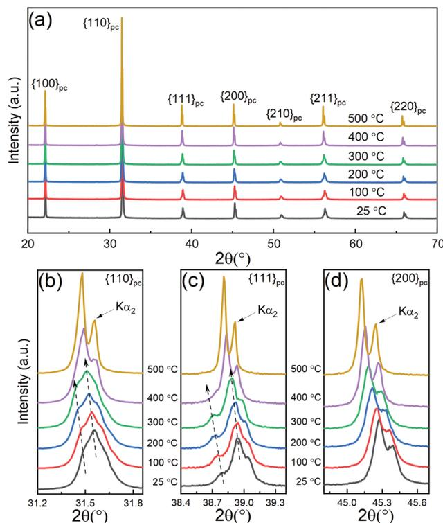
Fig. 1 (a) *In situ* XRD patterns of unpoled 0.5 mol% Nb-doped 0.7BF–0.3BT ceramics during heating. Details of the  $\{110\}_{\text{pc}}$ ,  $\{111\}_{\text{pc}}$  and  $\{200\}_{\text{pc}}$  peak profiles are shown in (b), (c) and (d) respectively. Arrow labels indicate the enhanced peak splitting of  $\{110\}_{\text{pc}}$  and  $\{111\}_{\text{pc}}$ , together with a gradual peak shift to lower angles due to thermal expansion, with increasing temperature.
