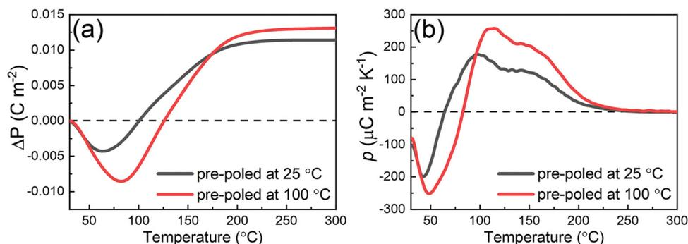
Fig. 6 Temperature-dependent changes in (a) remanent polarization,  $\Delta P$ , and (b) pyroelectric coefficient,  $p$ , of 0.5 mol% Nb-doped  $0.7\text{BF}$ – $0.3\text{BT}$  pre-poled at 25 and 100 °C.
