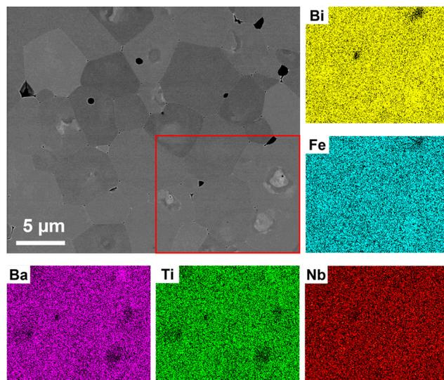
Fig. 3 SEM image (BSE mode) and EDS mapping of  $0.7\text{BiFeO}_3-0.3\text{Ba}(\text{Ti}_{0.995}\text{Nb}_{0.005})\text{O}_3$  ceramic. The core regions in the red rectangular area are relatively deficient in Ba and Ti but enriched in Bi and Fe.
