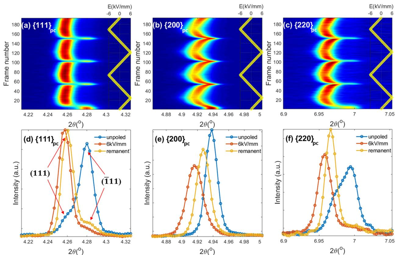
Fig. 7 Contour plots of Nb-doped 0.7BF-0.3BT ceramics at 125 °C of the  $\{111\}_{pc}$ ,  $\{200\}_{pc}$  and  $\{220\}_{pc}$  reflections under 2 bipolar electric field cycles in (a), (b) and (c) respectively, and comparison of peak profiles for the unpoled state, under 6 kV mm<sup>-1</sup> and in the remanent state in (d), (e) and (f).
