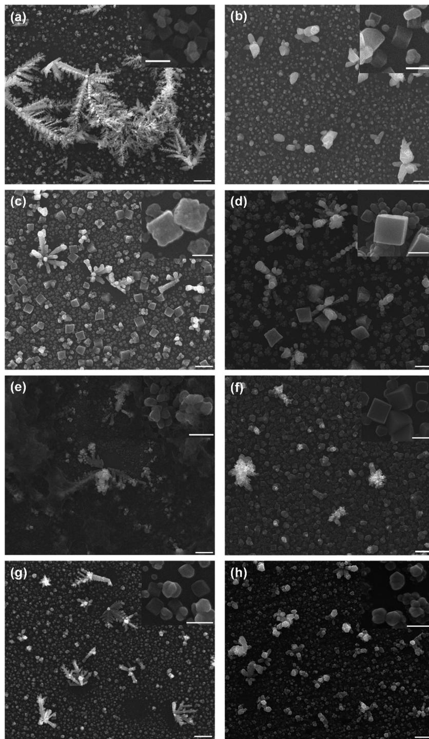
Fig. 7 Figure showing representative SEM images of (a and b) 5 mM  $\text{CuCl}_2$  with 5 mM NaCl, (c and d) 5 mM  $\text{Cu}(\text{CH}_3\text{CO}_2)_2$  with 5 mM NaCl, (e and f) 5 mM  $\text{Cu}(\text{NO}_3)_2$  with 5 mM NaCl, (g and h) 5 mM  $\text{CuSO}_4$  with 5 mM NaCl and 5 mM  $\text{Na}_2\text{SO}_4$ . (a, c, e and g) are from  $t_R > t_O$  depositions and (b, d, f and h) are from  $t_O > t_R$  depositions. Scale bars of images 1  $\mu\text{m}$ , insets 250 nm.
