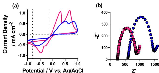
Fig. 1 Cyclic voltammograms (CVs) of 5 mM CuCl<sub>2</sub> in the presence of (blue) 5 mM and (pink) 50 mM NaCl using ITO-coated glass substrate as a working electrode, copper wire as a counter electrode and a Ag/AgCl (3 M NaCl) as a reference electrode. CVs were recorded with a scan rate of 50 mV s<sup>-1</sup>. Impedance was recorded in the same setup with an equilibrium potential of 0 V vs. the reference and an amplitude potential of 25 mV.
