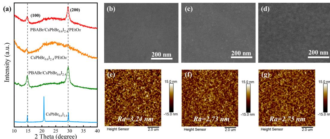
**Fig. 1** (a) Powder X-ray diffraction patterns of CsPbBr<sub>0.6</sub>I<sub>2.4</sub> thin films with different additives on glass substrates. (b–d) SEM images, and (e–g) AFM images showing the surface morphologies of CsPbBr<sub>0.6</sub>I<sub>2.4</sub> thin films with different additives at the same annealing temperature. From left to right: PBABr/CsPbBr<sub>0.6</sub>I<sub>2.4</sub>, CsPbBr<sub>0.6</sub>I<sub>2.4</sub>/PEtOx and PBABr/CsPbBr<sub>0.6</sub>I<sub>2.4</sub>/PEtOx.
