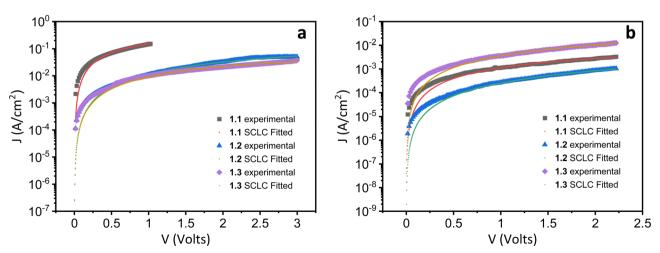
Fig. 3 Current density-voltage characteristics as a semi-log plot obtained for (a) hole and (b) electron mobilities extracted from SCLC devices in the thin film of compounds **1.1–1.3** at room temperature.
