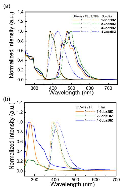
Fig. 5 (a) UV-vis absorption, fluorescence spectra in THF ( $10^{-5}$  M) and low temperature phosphorescence spectra in Me-THF ( $10^{-5}$  M) at 77 K; (b) UV-vis absorption and fluorescence spectra in thin films.
