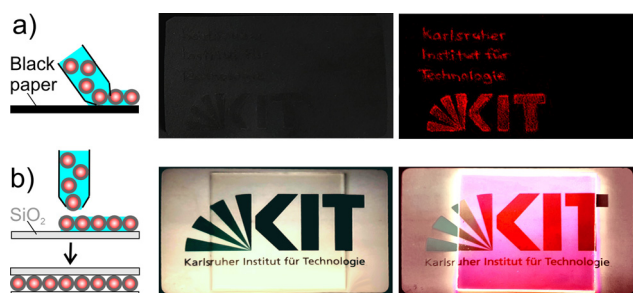
Fig. 8 Thin films with FR/CC@SiO 2 core-shell nanoparticles: (a) scheme of a pen filled with aqueous nanoparticle suspension and photos of written letters without and with excitation ( \lambda_{\text{exc}} = 366 nm), (b) scheme of nanoparticles between two quartz-glass plates and photos in daylight and with excitation ( \lambda_{\text{exc}} = 366 nm) (due to whitener the paper with the logo shows certain white emission itself).
