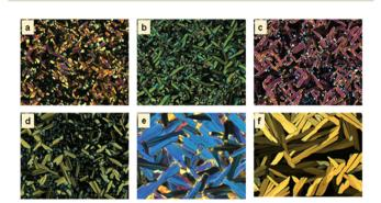
Fig. 3 POM microphotographs of the optical texture of Col phases formed by (a) P-5 at 280  $^{\circ}$ C, (b) P-6 at 230  $^{\circ}$ C, (c) P-7 at 225  $^{\circ}$ C, (d) P-8 at 190.7 °C, (e) **P-10** at 150.9 °C and (f) **P-11** at 214.9 °C.
