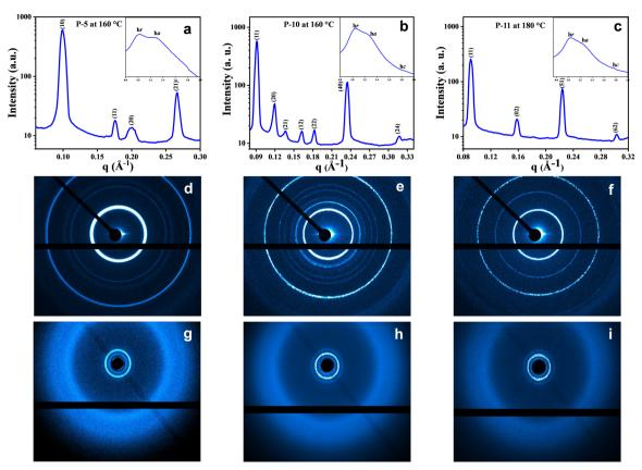
Fig. 4 Small- and wide-angle (inset) X-ray diffraction patterns of the Col phases formed by compounds (a) P-5 at 160 °C (Col<sub>n</sub>), (b) P-10 at 160 °C (Col<sub>ob</sub>) and (c) **P-11** at 180 °C (Col<sub>r</sub>) upon cooling (h<sub>r</sub>, cholesterol-cholesterol correlation; h<sub>a</sub>, alkyl chain-chain correlation; h<sub>c</sub>, disc-disc correlation). The lower panels show the respective 2D SAXS (d-f) and WAXS (g-i) diffraction patterns for the compounds in (a-c).
