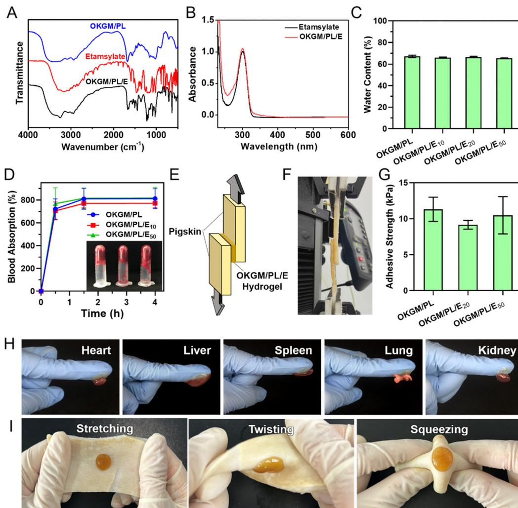
**Fig. 3** (A) FTIR spectra, (B) UV spectra, (C) water content, and (D) blood absorption of the OKGM/PL/E hydrogels. (E) Schematic illustration and (F) photograph of the lap shear experiment. (G) Adhesive strength of the OKGM/PL/E hydrogels. (H) and (I) Photographs showing the adhesion property of the OKGM/PL/E<sub>50</sub> hydrogels.
