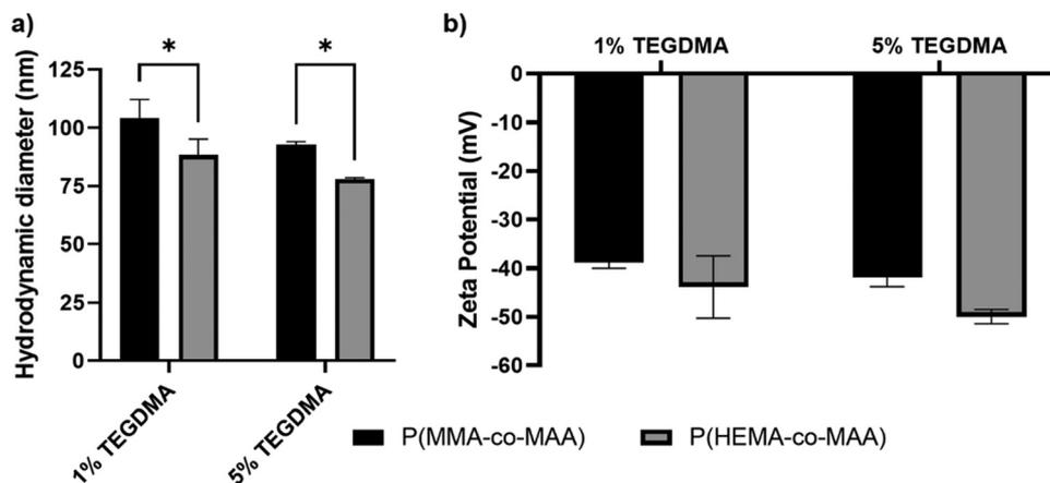
Fig. 2 (a) Hydrodynamic diameters and (b) zeta potential values of P(MMA-co-MAA) and P(HEMA-co-MAA) nanoparticles nominally crosslinked with 1 and 5 mol% TEGDMA. Hydrodynamic diameter measurements taken in 1 $\times$  PBS and zeta potential measurements taken in 5 mM sodium phosphate buffer, pH 7.4. \*  $p < 0.05$ .
