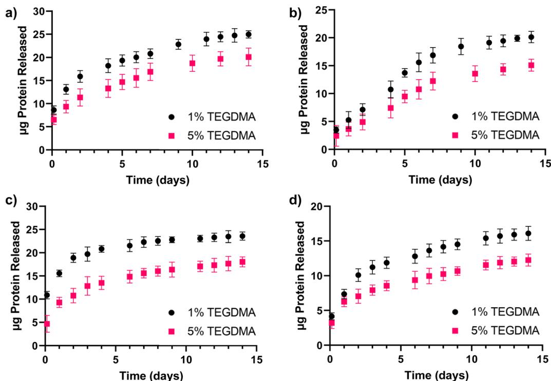
Fig. 7  $\alpha$ -Chymotrypsin release from P(MMA-co-MAA) nanoparticles covalently bound to (a) 2 and (b) 4 wt% chitosan scaffolds and P(HEMA-co-MAA) nanoparticles covalently bound to (c) 2 and (d) 4 wt% chitosan scaffolds in 1 $\times$  PBS at 37  $^{\circ}$ C, pH 7.4. Data shown are mean  $\pm$  SD ( $n = 3$ ).
