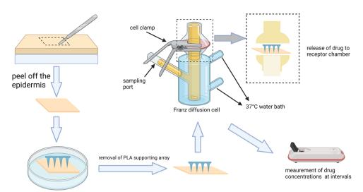
The procedure of using the Franz cell to determine the release property of MNs. This figure was adapted from the ref. 73.
