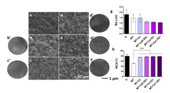
Fig. 2 SEM images of uncoated Ti (a), MT (b), MT-Ca (c), MT-Ca0.5Zn (d), MT-Ca1Zn (e), MT-Ca1.5Zn. Scale bars: (a-f) 10  $\mu$ m and (c'-f') 1  $\mu$ m. Profilometry measurements of the various sol-gel coatings and sandblasted Ti as a reference (g). Contact angle (WCA) results (h). The asterisk (\*) indicates differences between MT and the ion doped-samples; (\*\*\*) =  $p \le 0.001$ .
