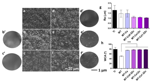
Fig. 2 SEM images of uncoated Ti (a), MT (b), MT-Ca (c), MT-Ca0.5Zn (d), MT-Ca1Zn (e), MT-Ca1.5Zn. Scale bars: (a–f) 10  $\mu\text{m}$  and (c'–f') 1  $\mu\text{m}$ . Profilometry measurements of the various sol-gel coatings and sandblasted Ti as a reference (g). Contact angle (WCA) results (h). The asterisk (\*) indicates differences between MT and the ion doped-samples; (\*\*\*) =  $p \leq 0.001$ .
