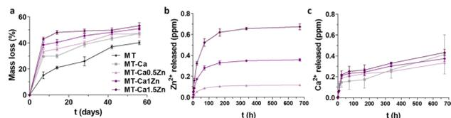
Fig. 3 (a) Sol-gel coatings hydrolytic degradation kinetic; (b) Zn<sup>2+</sup> and (c) Ca<sup>2+</sup> ions release from the various doped coatings. Data are represented as mean  $\pm$  SE.
