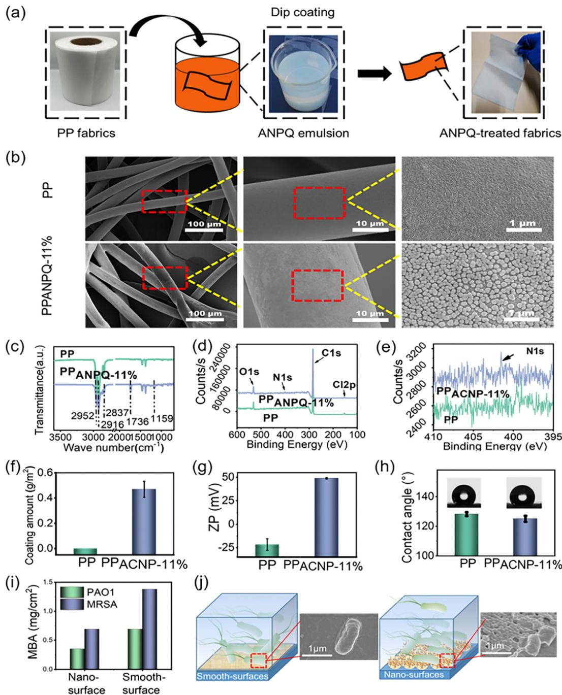
**Fig. 3** Characterization of ANPQ-11% coating. (a) Coating procedure and antibacterial mechanism of PP<sub>ANPQ-11%</sub>. Surface properties of PP and PP<sub>ANPQ-11%</sub>. (c) FTIR. (d and e) XPS. (f) Coating density. (g) Surface zeta potential. (h) Contact angle. (i) MBA against PAO1 and MRSA. (j) Scheme of bacteria touched with the surface coated with ANPQ.
