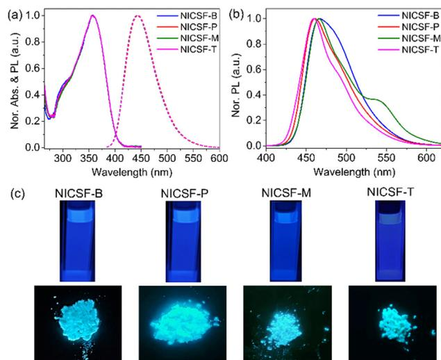
**Fig. 1** (a) The UV-vis absorption spectra (solid line) and PL spectra (dashed line) of NICSF-Xs in THF; (b) PL spectra (dashed line) of NICSF-Xs in the aggregated state; (c) the photos of NICSF-Xs in solution (upper row) and in powder (bottom row) irradiated under 365 nm UV light.
