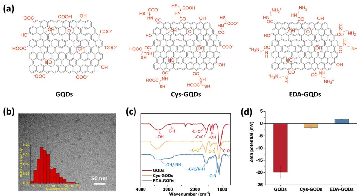
Fig. 1 (a) Molecular structure, (b) transmission electron microscope (TEM) image and size distribution of GQDs. The average diameter is  $8.1 \pm 2.5$  nm. (Scale bar: 50 nm.) (c) Fourier transform infrared (FTIR) spectra and (d) zeta potentials of GQDs, Cys-GQDs, and EDA-GQDs.
