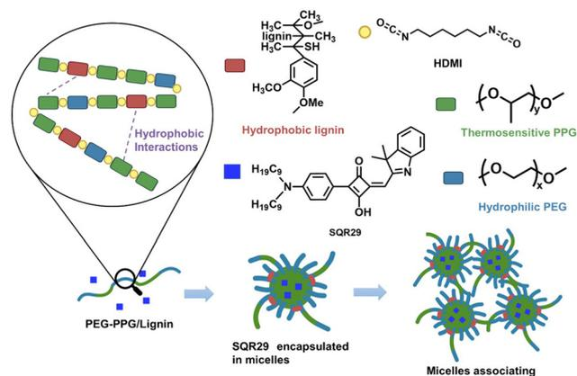
Fig. 1 Schematic representation of the micelle association model between Lignin-PEG-PPG and SQR29.
