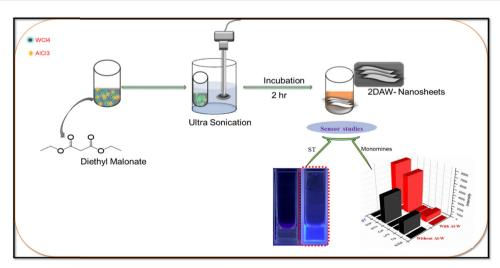
Fig. 1 Schematic presentation to show the reaction procedures for the preparation of Al-W nanosheets and sensor studies for the detection of serotonin with the selectivity 3D graph.
