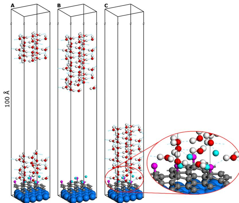
**Fig. 1** The simplified sketch of the ice/graphene bilayer computational models used for the determination of the cohesion (A and C) and adhesion (B and C) energies. The insert shows the details of the interface geometry. Functional groups are colored differently for clarity (oxygen – magenta, hydrogen – cyan). For the same purpose, the ice slab thickness was also decreased.
