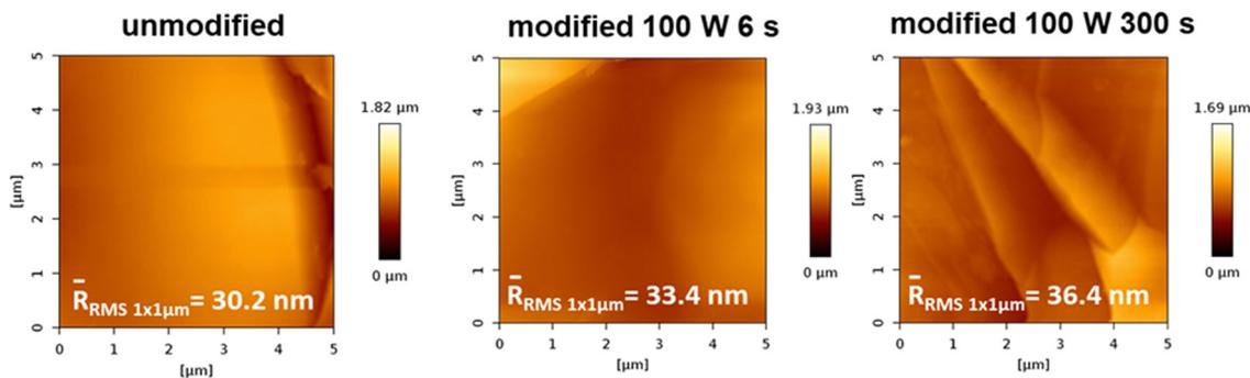
Fig. 3 Representative AFM images of the unmodified and oxygen-plasma modified graphenic surfaces together with the averaged  $\bar{R}_{\text{RMS}}$  values were determined for the basal plane  $1 \mu\text{m}^2$  area, illustrating surface structure stability upon exposure to plasma under the applied conditions.
