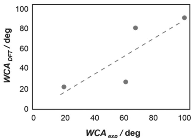
**Fig. 9** The correlation between experimentally measured and theoretically determined water contact angle values.
