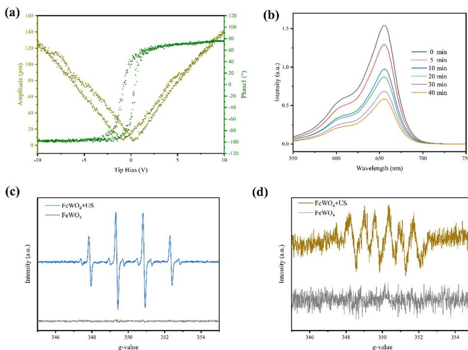
Fig. 2 Piezocatalytic performance under US irradiation. (a) Piezo-response of phase curve and amplitude curve of  $\text{FeWO}_4$  nanorods. (b) Degradation of MB with different US irradiation time in the presence of  $\text{FeWO}_4$ . ESR spectra of  $\cdot\text{OH}$  (c) and  $\cdot\text{O}_2^-$  (d) under US irradiation.
