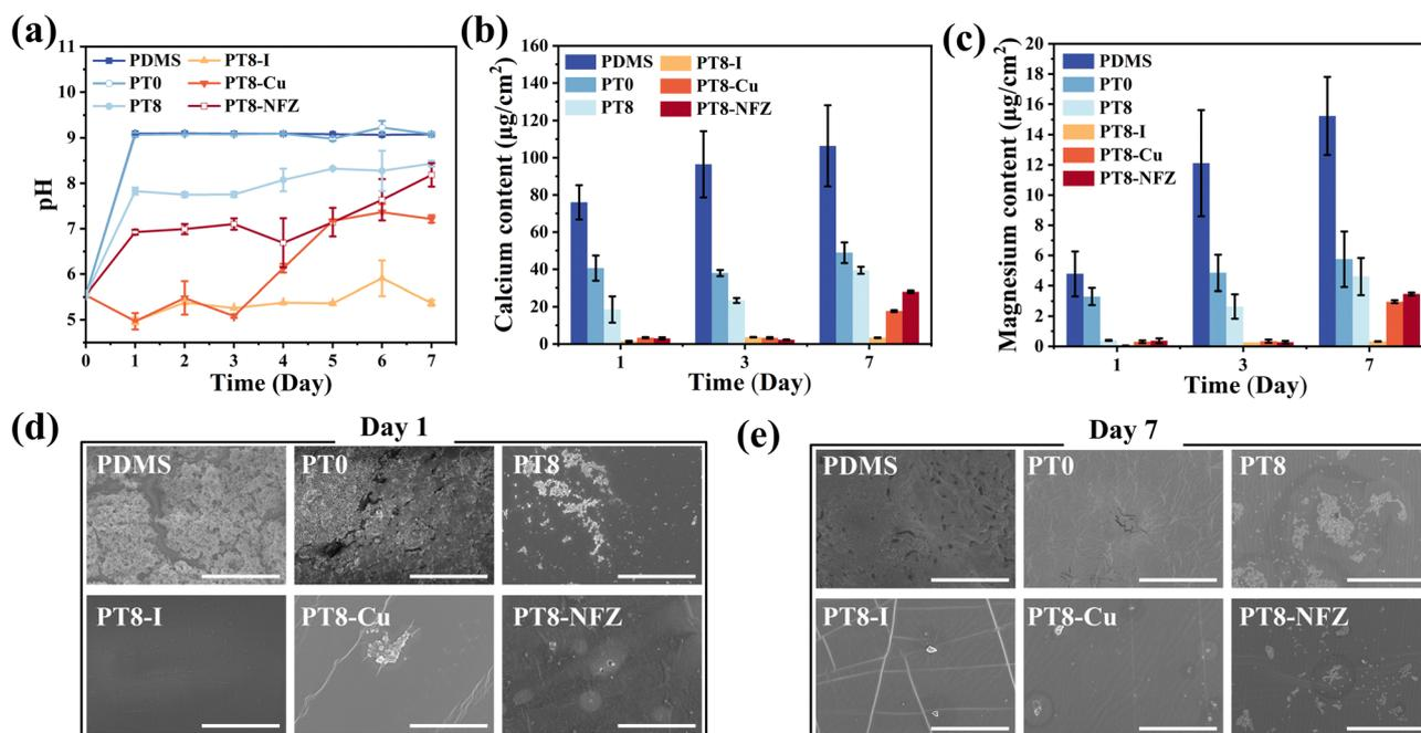
Fig. 4 (a) Change in pH value of artificial urine inoculated with  $10^5$  CFU per mL of *P. mirabilis* containing pristine and modified PDMS substrate over 7 days. The content of (b) calcium and (c) magnesium elements deposited on the surface of pristine and modified PDMS after incubating in artificial urine containing *P. mirabilis* over 7 days. SEM images of pristine and modified PDMS surfaces after an encrustation test for (d) 1 day and (e) 7 days. Scale bars represent 50  $\mu\text{m}$ .
