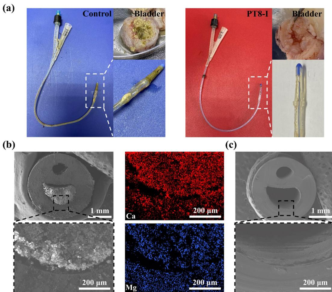
Fig. 6 (a) Photographs of a catheter and rabbit bladder harvested from an animal after implantation for 7 days. (b) SEM images and EDS mapping of cross-section of unmodified catheter after implantation for 7 days. (c) SEM images of cross-section of PT8-I-coated catheter after implantation for 7 days.
