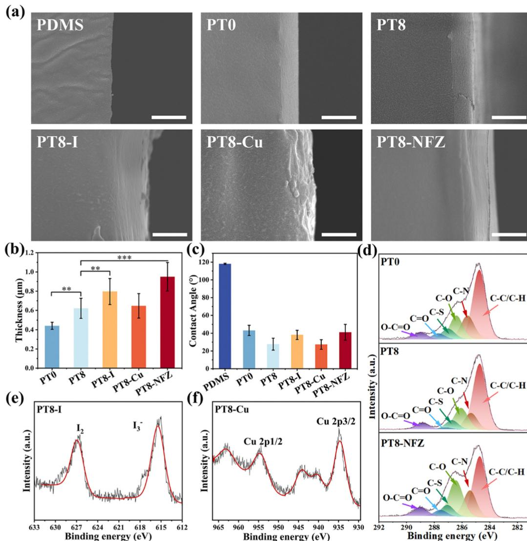
Fig. 1 (a) SEM images of the cross-section of pristine and modified PDMS. Scale bars represent 1  $\mu\text{m}$ . (b) Thickness of hydrogel coating on PDMS. (c) Water contact angles of pristine and modified PDMS surfaces. (d) C 1s, (e) I 3d, and (f) Cu 2p core-level XPS spectra of modified PDMS surfaces.
