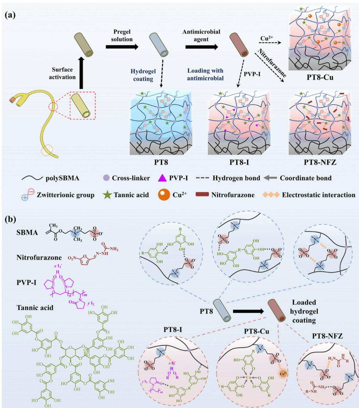
**Scheme 1** Schematic diagram illustrating (a) the preparation process of a multifunctional hydrogel coating on a urinary catheter surface, and (b) the structure of PT8 hydrogel coating, and antimicrobial-loaded hydrogel coating (i.e. PT8-I, PT8-Cu, and PT8-NFZ).
