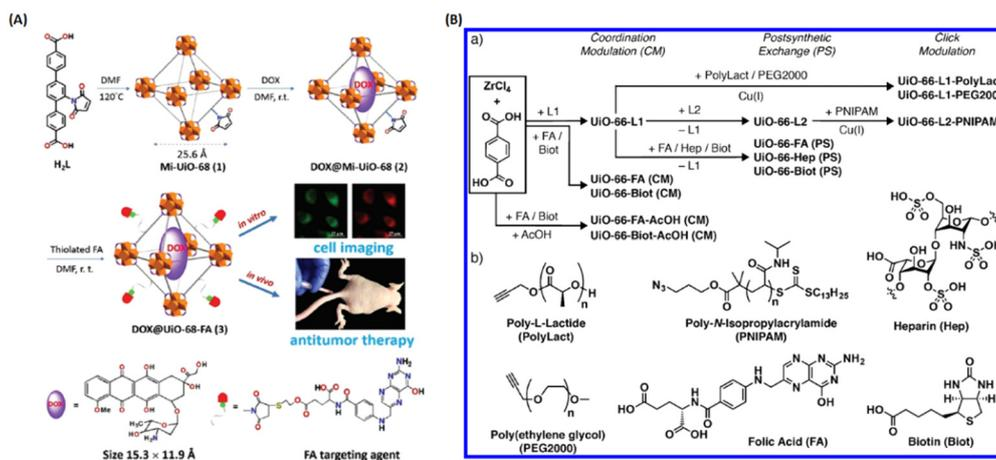
Fig. 5 Covalent attachment of targeting agents to MOFs for targeted delivery. (A) Design and fabrication of FA targeting agent-decorated drug delivery system and its application in cell imaging and *in vivo* antitumor therapy.<sup>31</sup> Copyright 2016, Chemical Communications (Camb). (B) Synthetic scheme for the three surface-modified protocol of UiO-66 and the attachment of chemical structures.<sup>28</sup> Copyright 2018, *ACS Applied Materials & Interfaces*.
