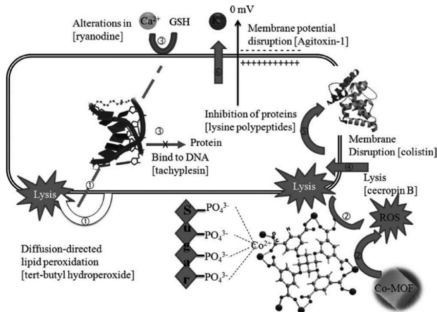
Fig. 21 The mechanism of bactericidal activities using Co-TDM single crystals as disinfectants: six steps synergistically contribute to the bactericidal efficacy.<sup>170</sup> Copyright 2012, *Advanced Healthcare Materials*.
