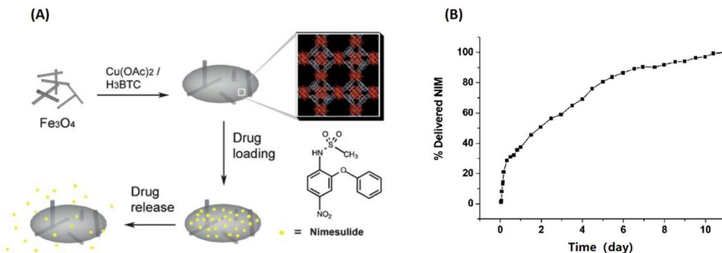
Fig. 4 Fe<sub>3</sub>O<sub>4</sub>@MOF for magnetic targeted drug delivery and controlled release. (A) The synthesis and action of Fe<sub>3</sub>O<sub>4</sub>/Cu<sub>3</sub>(BTC)<sub>2</sub> nanocomposites for potential targeted drug release; (B) the NIM release process in physiological saline at 37 °C.<sup>29</sup> Copyright 2011, *Journal of Materials Chemistry*.
