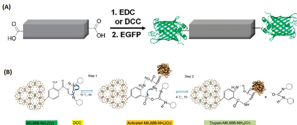
Fig. 11 The bioconjugation of proteins onto the surface of MOFs *via* functional groups of the organic linkers. (A) The bioconjugation of the 1D-MOFs,  $[(\text{Et}_2\text{NH}_2)(\text{In}(\text{pda})_2)]_n$ , with EGFP.<sup>89</sup> Copyright 2011, Chemical Communications (Camb). (B) Trypsin immobilization onto DCC-activated MIL-88B-NH<sub>2</sub>(Cr).<sup>90</sup> Copyright 2012, *ChemPlusChem*.
