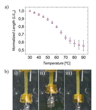
Fig. 2 Thermomechanical response in PBS buffer of uniaxial oriented LCEs (65  $\pm$  5  $\mu m$  thick) with the director along its long axis. A load of 1 g attached to the extreme of the samples is lifted upon actuation. (a) Normalized length  $(L/L_0)$  of the LC elastomers during the heating from 30 °C to 90 °C. Mean  $\pm$  SD of two samples. (b) Camera images collected at (i) 30 °C to (ii) 90 °C and after cooling down (iii) at 30 °C. Scale bar represents 5 mm.
