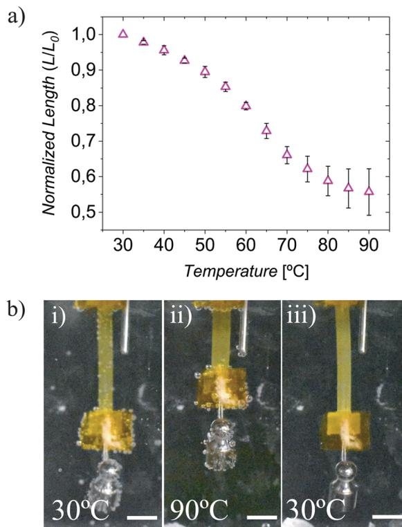
Fig. 2 Thermomechanical response in PBS buffer of uniaxially oriented LCEs ( $65 \pm 5 \mu\text{m}$  thick) with the director along its long axis. A load of 1 g attached to the extreme of the samples is lifted upon actuation. (a) Normalized length ( $L/L_0$ ) of the LC elastomers during the heating from 30 °C to 90 °C. Mean  $\pm$  SD of two samples. (b) Camera images collected at (i) 30 °C to (ii) 90 °C and after cooling down (iii) at 30 °C. Scale bar represents 5 mm.
