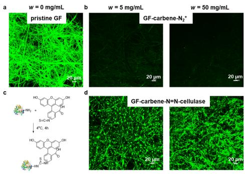
Fig. 6 Visualization of FITC-labelled surface using confocal microscope: (a) pristine **GF membrane**, (b) **GF-carbene-N<sub>2</sub>**<sup>+</sup> with w = 5 mg mL<sup>-1</sup> and 50 mg mL<sup>-1</sup>, (c) schematic illustration of FITC with cellulase, (d) **GF-carbene-N—N-cellulase** with w = 5 mg mL<sup>-1</sup> and 50 mg mL<sup>-1</sup>
