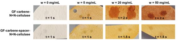
Fig. 2 Images of water droplet on surfaces at different bis(diarydiazomethane) concentration after fully wetted, and the time taken for the water droplet to fully wet the surface has been labelled (unit: s).
