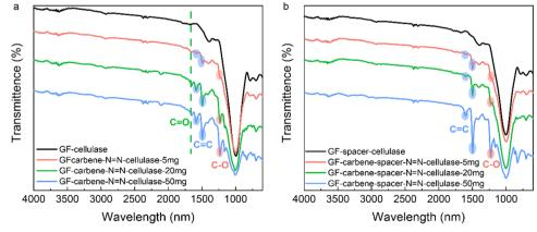
Fig. 4 ATR-IR of (a) immobilized cellulase on membranes of GF modified with bis(diarylcarbene) at different concentration; (b) immobilized cellulase on membrane of GF modified with bis(diarylcarbene) at different concentration plus spacer addition.
