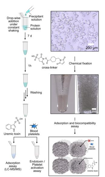
Fig. 2 Schematic overview of batch crystallization technique for fabrication of protein-based adsorption materials, images of the material before and after fixation and schematic depiction of the size-exclusion effect for excluding blood platelets from the inner cavity.
