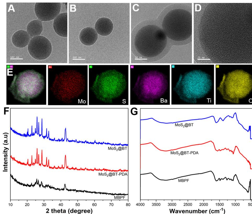
**Fig. 1** Structure, morphological and chemical composition of CSNPs. TEM images of (A) and (B) the spherical-shaped group of CSNPs, (C) and (D) the morphology of the shell at higher magnification, (E) EDX mapping of  $\text{MoS}_2$ @BT CSNPs, (F) XRD and (G) FT-IR spectra of  $\text{MoS}_2$ @BT,  $\text{MoS}_2$ @BT-PDA, and MBPF CSNPs.
