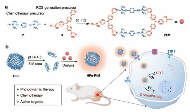
Scheme 1 (a) Schematic of the synthesis of an organoplatinum(II) metallacycle PtM. (b) Schematic illustration of the preparation of the HFn-PtM targeted chemo-photodynamic combination therapy after intravenous (i.v.) injection under light irradiation.
