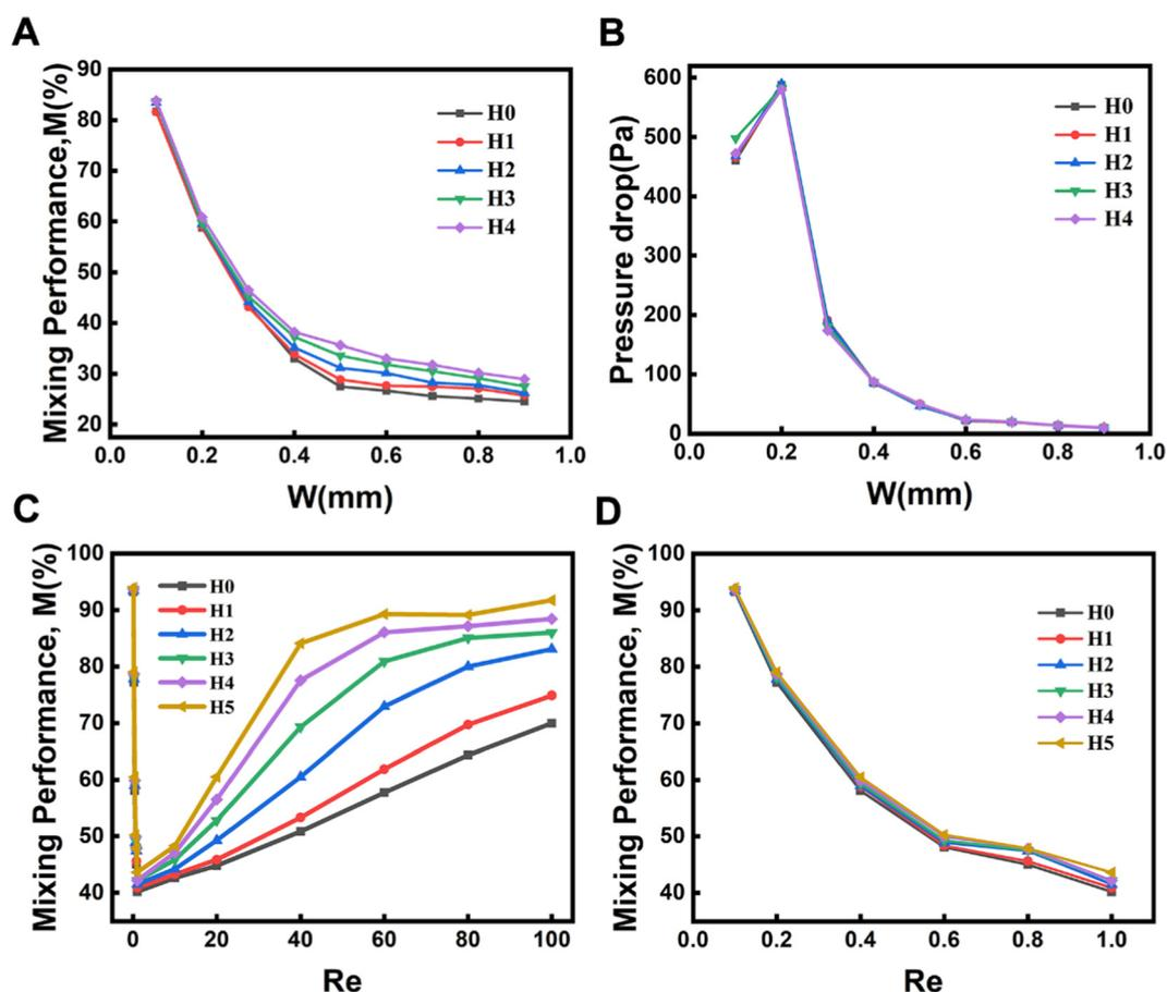
Fig. 3 Influencing factors of mixing performance. Effect of channel width on the mixing efficiency (A) and pressure drop (B). Mixing efficiency comparison of six hyperbolic curves in  $Re$  from 0.1 to 100 (C) and 0.1 to 1.0 (D).
