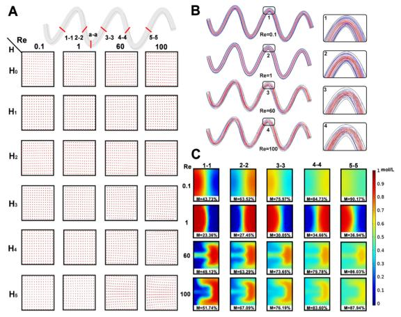
Fig. 4 (A) Flow direction of six hyperbolic curves of the micromixer at different Re for the cross-sections. (B) Streamlining of the hyperbolic micromixer's curve  $H_5$  micromixer at different Re and amplified view at channel and curves. (C) Concentration distribution of the cross-section of the hyperbolic curve H<sub>5</sub> of the micromixer at different Re.
