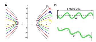
Fig. 1 (A) Schematic diagram of six hyperbolas. (B) Schematic diagram of a hyperbolic micromixer.
