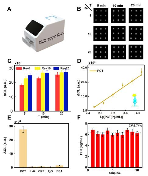
Fig. 6 (A) Chemiluminescence detection apparatus, PCT concentration of 3.2 ng mL<sup>-1</sup> at different Re and incubation times for dot signal (B) and corresponding  $\Delta$ CL intensity (C). (D) Standard curve between the PCT concentration and  $\Delta$ CL intensity (N = 3). (E) The selectivity assay of the developed for detection of PCT. (F) The stability research of the chips (No. 10) for PCT (6.4 ng mL<sup>-1</sup>) analysis.
