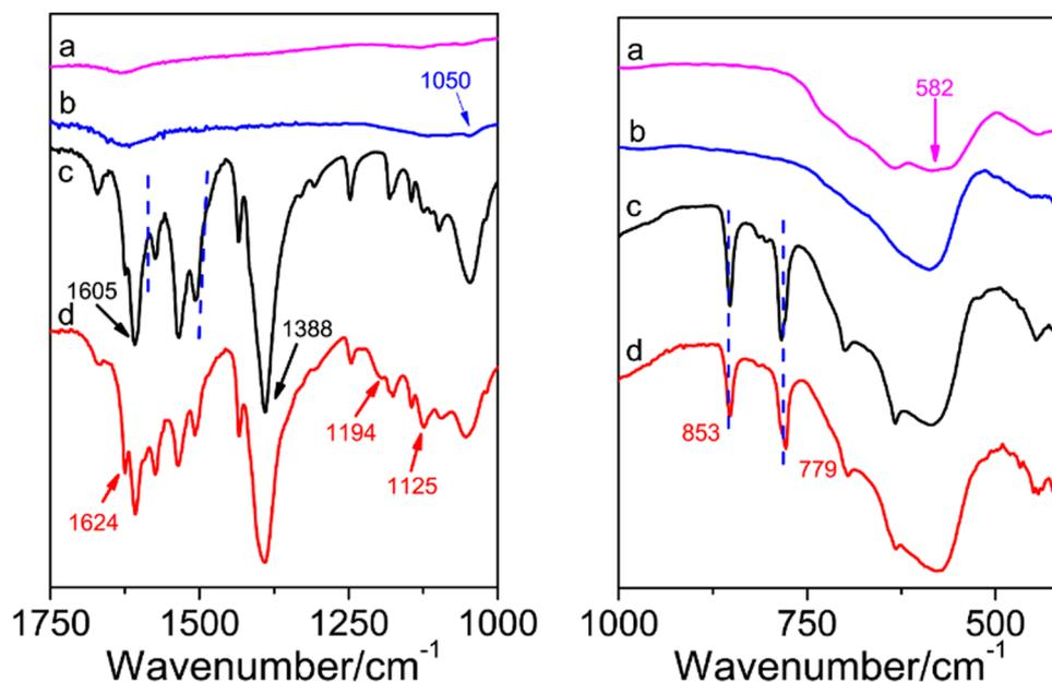
Fig. 1 FTIR spectra of (a) Fe<sub>3</sub>O<sub>4</sub>, (b) Fe<sub>3</sub>O<sub>4</sub>@PDA, (c) Fe<sub>3</sub>O<sub>4</sub>@MOF, and (d) ILs/Fe<sub>3</sub>O<sub>4</sub>@MOF.
