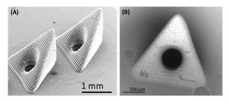
Fig. 2 Illustration of SEM image of (A) hollow microneedle array and (B) single hollow microneedle
