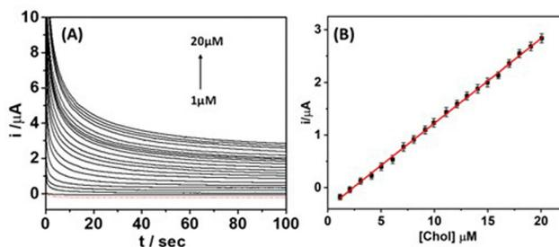
Fig. 3 (A) Chronoamperometric response of the microneedle sensor toward increasing concentrations of cholesterol (1  $\mu\text{M}$  increments) in PBS solution over a 1–20  $\mu\text{M}$  range; the potential was applied at +0.65 V (*vs.* Ag/AgCl). (B) The respective calibration plots for up to 20  $\mu\text{M}$  cholesterol based on sampling the current at 100 s.
