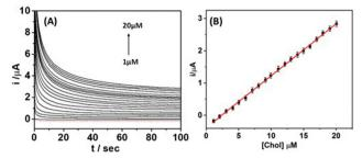
Fig. 3 (A) Chronoamperometric response of the microneedle sensor toward increasing concentrations of cholesterol (1  $\mu M$  increments) in PBS solution over a 1–20  $\mu$ M range; the potential was applied at +0.65 V (vs. Ag/AgCl). (B) The respective calibration plots for up to 20  $\mu M$  cholesterol based on sampling the current at 100 s.
