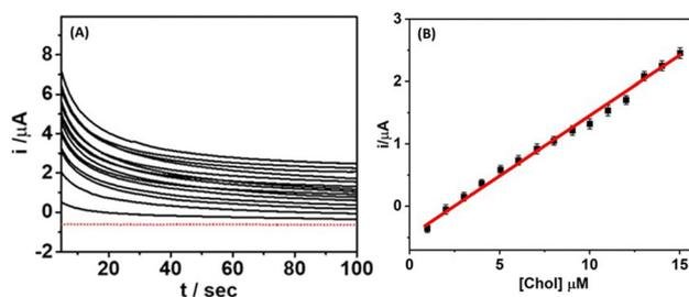
Fig. 4 (A) Chronoamperometric response of the microneedle sensor toward increasing concentrations of cholesterol (1  $\mu\text{M}$  increments) in an artificial interstitial fluid sample over the 1–15  $\mu\text{M}$  range; potential applied at +0.65 V (*vs.* Ag/AgCl). (B) The respective calibration plots up to 15  $\mu\text{M}$  cholesterol based on sampling the current at 100 s.
