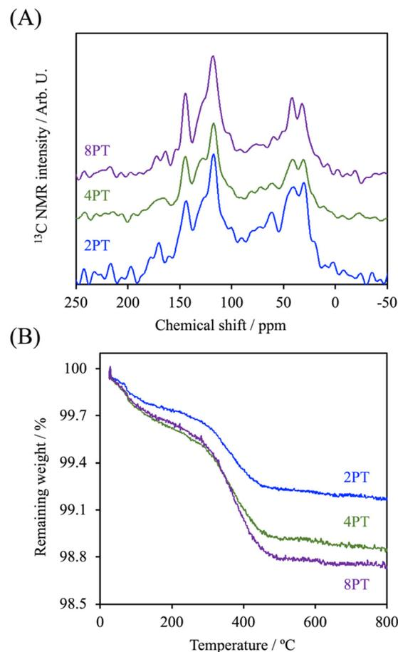
Fig. 2 (A) <sup>13</sup>C ssNMR spectra and (B) TGA curve of PDA- $\beta$ -TCP synthesized at different concentrations of the DA precursor.
