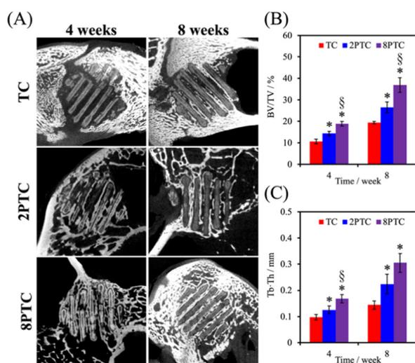
Fig. 9 (A)  $\mu$ -CT images of bone defects implanted with different scaffolds for 4 and 8 weeks. (B) Bone volume fraction (BV/TV) and (C) trabecular thickness (Tb.th) in different scaffolds. \* and § indicate significant differences ( $p < 0.05$ ) compared to TC and 2PTC, respectively.
