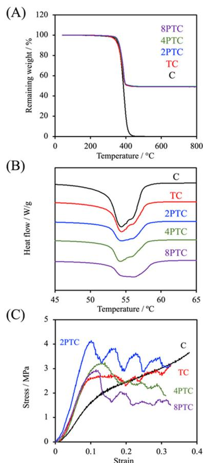
Fig. 5 (A) TGA, (B) DSC, and (C) compressive stress–strain curves of different scaffolds.
