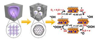
Thin carbon layer covered  $Co_4N$  cubes encapsulated in N-doped porous carbon nanocage as trifunctional catalysts with enhanced charge-transfer efficiency for Zn-air battery and overall watersplitting
