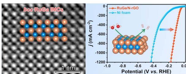
**Atomically dispersed ruthenium sites with electron-rich environments in intermetallic compounds for high-current-density hydrogen evolution**
