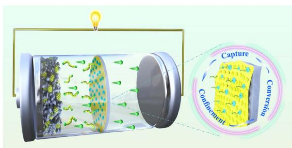
**Developing a MXene quantum dot-based separator for Li-S batteries**
