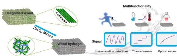
**Construction of MXene functionalized wood-based hydrogels using  $ZnCl_2$  aqueous solution for flexible electronics**
