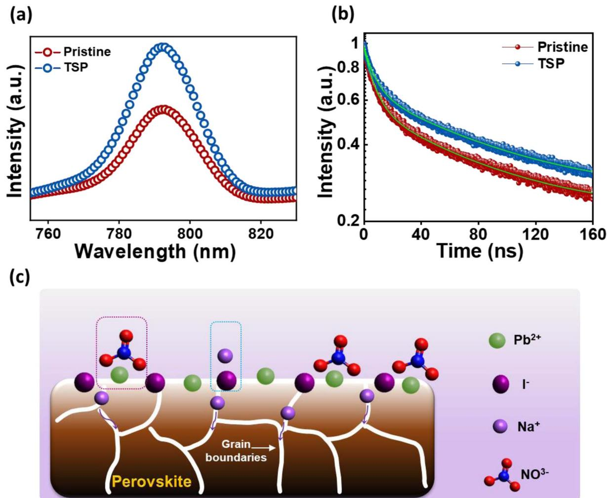
Fig. 4 (a) PL spectra for pristine and TSP films. (b) TRPL spectra for pristine and TSP films. (c) Probable mechanism for interaction of NaNO<sub>3</sub> at the perovskite/ETL interface.
