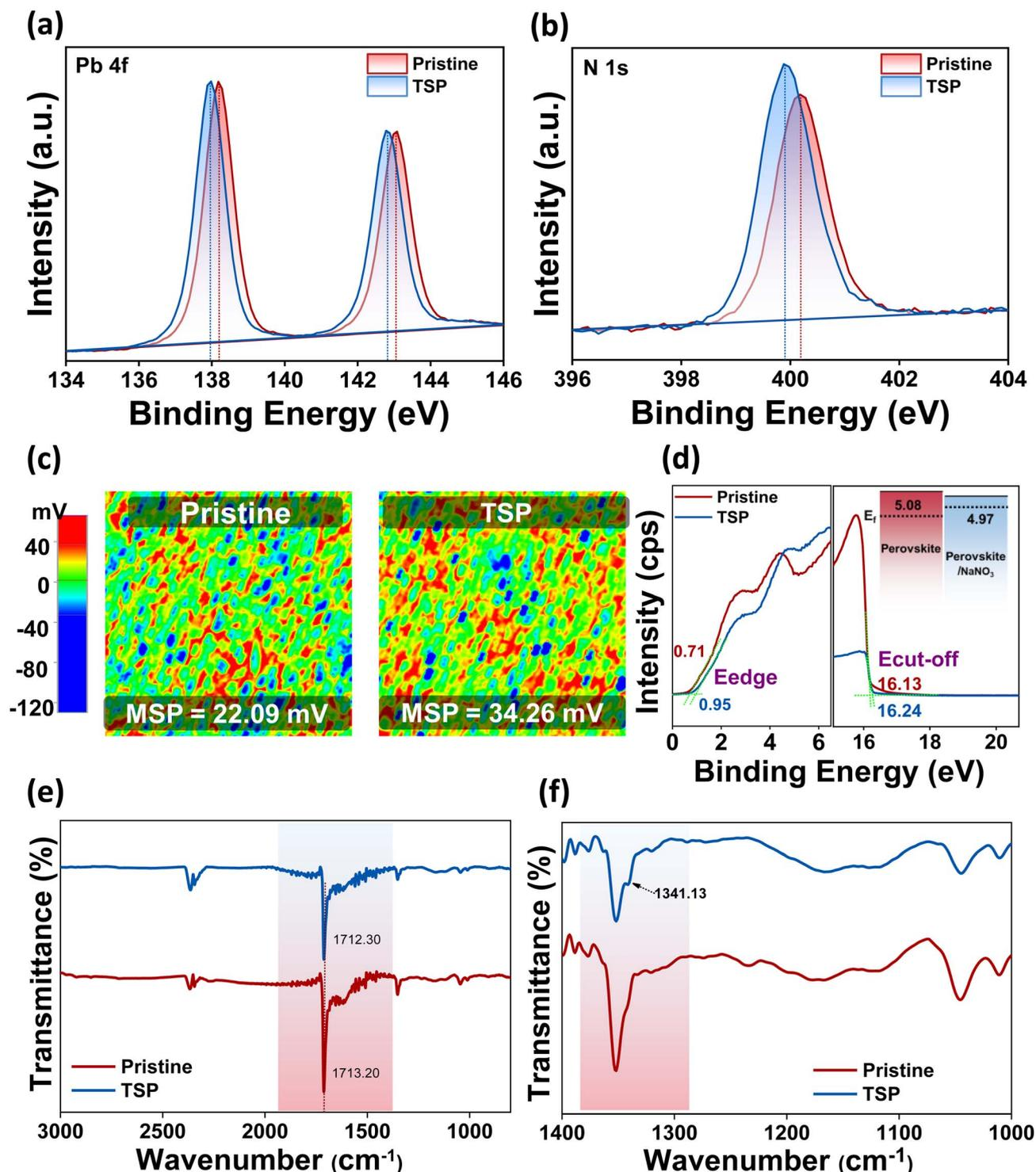
Fig. 3 X-ray photoelectron spectroscopy (XPS) spectra of (a) Pb 4f and (b) N 1s. (c) Scanning Kelvin probe microscopy (SKPM) images of pristine and TSP perovskite films. (MSP = mean surface potential). (d) UPS spectra of the perovskite and TSP films (inset shows energy level alignment). (e) FTIR spectra of pristine and TSP films. (f) FTIR spectra of pristine and TSP in the expanded fingerprint region for 1400–1000 cm<sup>-1</sup>.
