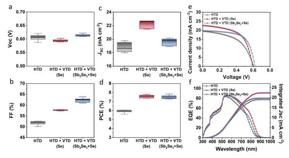
Fig. 2 Device performance of HTD, HTD + VTD (Se), and HTD + VTD (Sb<sub>2</sub>Se<sub>3</sub> + Se) Sb<sub>2</sub>(S,Se)<sub>3</sub> solar cells: Statistical box plots of (a)  $V_{oc}$ , (b) FF, (c)  $J_{sc}$ , (d) PCE, (e) J-V curves, and (f) EQE spectra.
