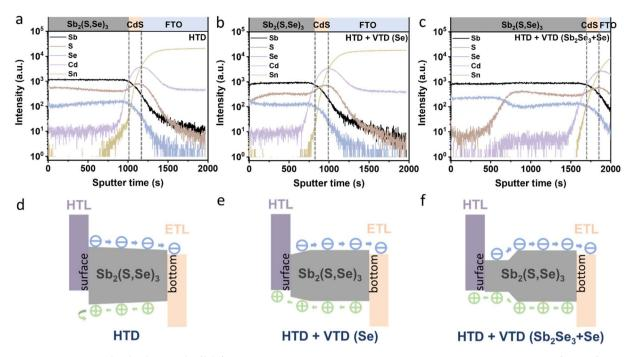
Fig. 4 Depth profiling via TOF-SIMS of the Sb<sub>2</sub>(S,Se)<sub>3</sub> films and energy band structures of the corresponding solar devices: (a and d) HTD, (b and e) HTD + VTD (Se), and (c and f) HTD + VTD (Sb<sub>2</sub>Se<sub>3</sub> + Se).
