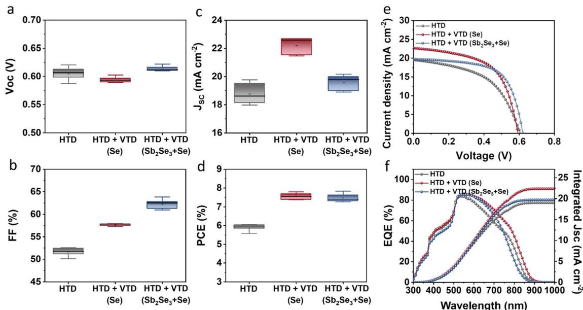
Fig. 2 Device performance of HTD, HTD + VTD (Se), and HTD + VTD ( $\text{Sb}_2\text{Se}_3 + \text{Se}$ )  $\text{Sb}_2(\text{S,Se})_3$  solar cells: Statistical box plots of (a)  $V_{oc}$ , (b) FF, (c)  $J_{sc}$ , (d) PCE, (e)  $J-V$  curves, and (f) EQE spectra.
