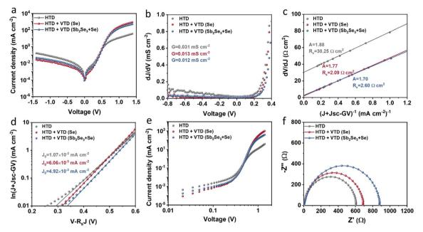
Fig. 5 Charge transport behaviors of the representative  $Sb_2(S,Se)_3$  devices: (a) semi-logarithmic dark J-V plots, (b)  $dJ dV^{-1}$  versus V plots for G, (c) dV/dJ versus ( $J + J_{sc} - GV$ ) plots for extracting  $R_s$  and A, (d)  $\ln(J + J_{sc} - GV)$  versus  $V - R_sJ$  plots for extracting  $J_0$ , (e) SCLC spectra derived from the dark J-V curves, and (f) Nyquist plots extracted from IS.
