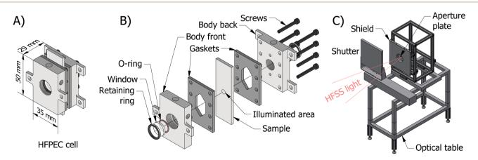
Fig. 1 An overview of the experimental setup: (A) CAD diagram of the assembled HFPEC cell, (B) CAD diagram of disassembled cell highlighting each layer, and (C) the experimental setup at the high flux solar simulator (HFSS) facility highlighting key components.
