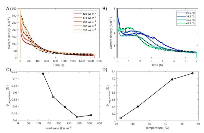
Fig. 7 Results of the model for prediction of BiVO<sub>4</sub> degradation. Experimental and predicted photocurrent densities at (A) different irradiances,  $122-358 \text{ kW m}^{-2}$ , and (B) different temperatures  $26-48 \,^{\circ}\text{C}$ , under  $1 \, \text{sun} = 1 \, \text{kW m}^{-2}$ . (C) Estimated fraction of current towards degradation viadissolution of BiVO<sub>4</sub> as a function of (C) irradiance and (D) temperature.
