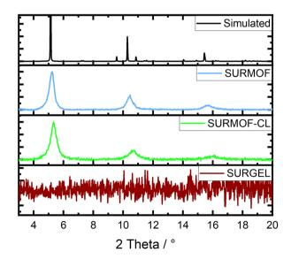
Fig. 3 (a) Importance of variables for the five chosen variables c (linker), c (metal), modulator (water), DABCO (additive) and ethanol (solvent) in relative values between 0 and 1. (b) XRD of SURMOF, SURFMOF-CL and SURGEL.
