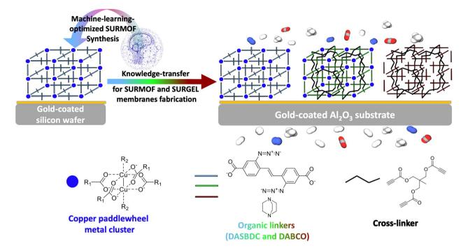
Fig. 1 Schematic overview of the development of membranes for gas separation. First the SURMOF is optimized *via* machine learning on gold coated silicon wafers, then the optimized conditions are transferred on gold coated alumina substrates to fabricate a SURMOF, a crosslinked SURMOF and a SURGEL for gas separation investigation.
