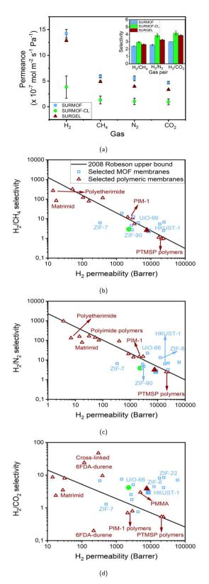
Fig. 4 (a) Gas permeance and gas selectivity (inset) of SURMOF, SURMOF-CL and SURGEL membranes. (b)  $H_2/CH_4$ , (c)  $H_2/N_2$  and (d) H<sub>2</sub>/CO<sub>2</sub> gas separation performance comparisons of SURMOF, SUR-MOF-CL and SURGEL membranes against selected membranes<sup>30,54–65</sup> and polymeric membranes.<sup>4,66–88</sup> The legends in the figures (a) and (b) apply for all the figures
