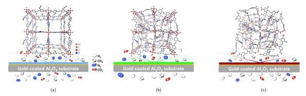
Fig. 5 Illustration of the unit cell and the membrane performance of the SURMOF (a), SURMOF-CL (b) and SURGEL (c).
