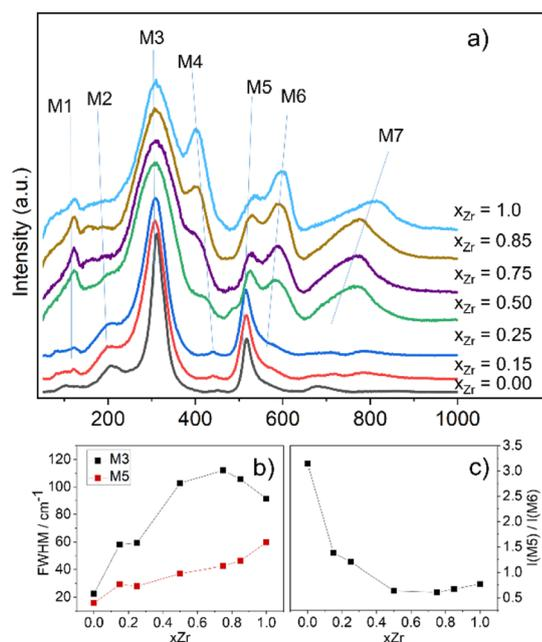
Fig. 3 Raman spectra of  $Gd_2(Ti_{1-x}Zr_x)_2O_7$  series between 50 and  $1000\text{ cm}^{-1}$  (a) offset on the Y axis. After background subtraction, each spectrum was normalized between 0 and 100; FWHM of modes M3 and M5 (b) and intensity ratio between modes M5 and M6 (c) as a function of Zr-content.
