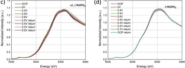
Fig. 9 In situ Ni K-edge XANES spectra of (a)  $\alpha$ -Ni(OH)<sub>2</sub>, (b)  $\alpha\beta$ \_1-Ni(OH)<sub>2</sub>, (c)  $\alpha\beta$ \_2-Ni(OH)<sub>2</sub> and (d)  $\beta$ -Ni(OH)<sub>2</sub> under a oxidation and reduction scans.
