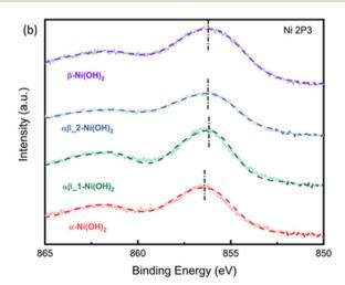
(a) XPS survey spectrum of nickel hydroxide (b) Ni 2p XPS spectra of nickel hydroxide of different phases.
