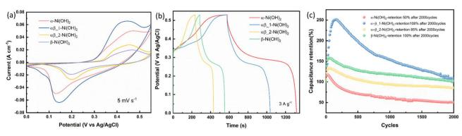
Fig. 7 (a) CV curves at 5 mV s $^{-1}$ . (b) GCD curves at 3 A g $^{-1}$ . (c) Cycling performance for different nickel hydroxide samples in the three-electrode configuration.
