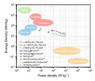
Fig. 12 Ragone plot of Ni(OH)<sub>2</sub>//AC hybrid supercapacitors.<sup>46–51</sup>
