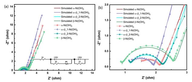
(a) Nyquist plots, inset show the corresponding equivalent circuit of different electrodes of nickel hydroxide. (b) The enlarged Nyquist plots.
