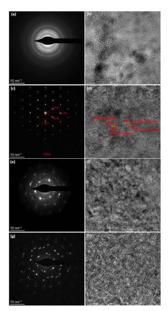
Fig. 2 (a and b) HRTEM Images of  $\alpha$ -Ni(OH)<sub>2</sub> with SAED pattern. (c and d) HRTEM images of  $\beta$ -Ni(OH)<sub>2</sub> with SAED pattern. (e and f) HRTEM images of  $\alpha\beta_1$ -Ni(OH)<sub>2</sub> with SAED pattern. (g and h) HRTEM images of  $\alpha\beta_2$ -Ni(OH)<sub>2</sub> with SAED pattern.
