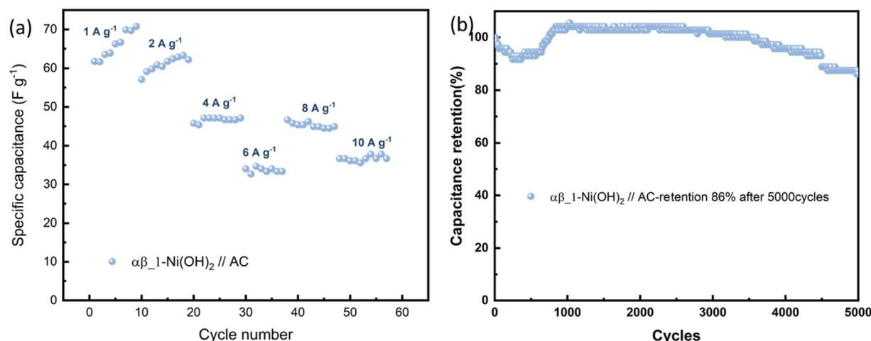
Fig. 11 (a) The specific capacitance evolution under various current densities of  $\alpha\beta_1$ -Ni(OH)<sub>2</sub>//AC. (b) Cycling performance at 100 mA cm<sup>-1</sup> for 5000 cycles.
