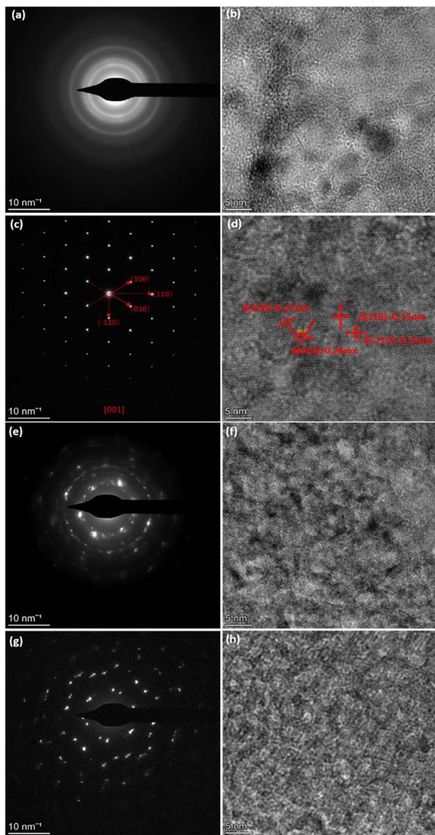
Fig. 2 (a and b) HRTEM Images of  $\alpha$ -Ni(OH)<sub>2</sub> with SAED pattern. (c and d) HRTEM images of  $\beta$ -Ni(OH)<sub>2</sub> with SAED pattern. (e and f) HRTEM images of  $\alpha\beta$ \_1-Ni(OH)<sub>2</sub> with SAED pattern. (g and h) HRTEM images of  $\alpha\beta$ \_2-Ni(OH)<sub>2</sub> with SAED pattern.
