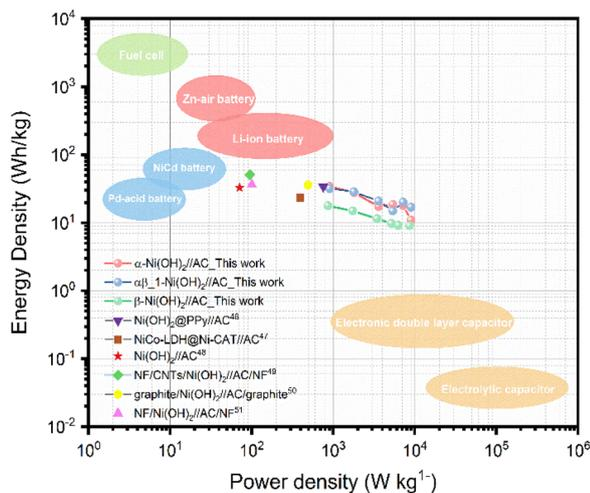
Fig. 12 Ragone plot of  $\text{Ni}(\text{OH})_2//\text{AC}$  hybrid supercapacitors.<sup>46–51</sup>
