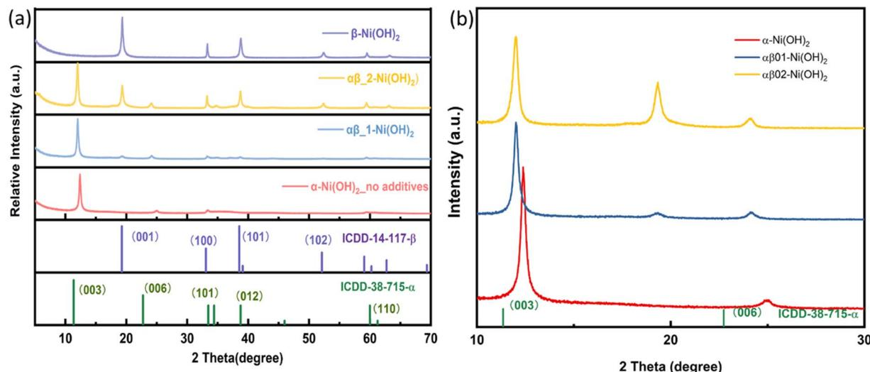
Fig. 1 (a) PXRD patterns of nickel hydroxide powder prepared with additive  $\text{NH}_4\text{F}$ . (b) Expanded 2 theta region of PXRD patterns highlighting the 003 and 006 reflections of the alpha phase for  $\alpha\text{-Ni(OH)}_2$ ,  $\alpha\beta_1\text{-Ni(OH)}_2$ ,  $\alpha\beta_2\text{-Ni(OH)}_2$ .
