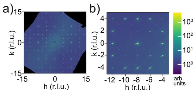
Fig. 6 (a) Synchrotron single crystal scattering pattern for Li<sub>5.5</sub>-LLNZO in the *hk0* plane. (b) Enlarged region of *hk0* scattering plane showing additional Bragg reflections in *hk0* with  $h + k = 2n$  and in *h00* or *0k0* with  $h$  or  $k = 4n + 2$ .
