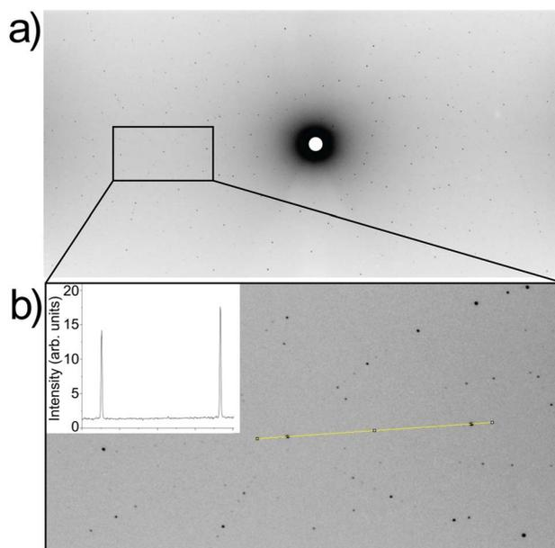
Fig. 4 (a) Representative Laue neutron diffraction image for Li<sub>5.5</sub>-LLNZO. (b) Enlarged area indicated in (a). Intensity profile through several selected reflections highlighted in yellow is shown in inset, illustrating high crystal and data quality.
