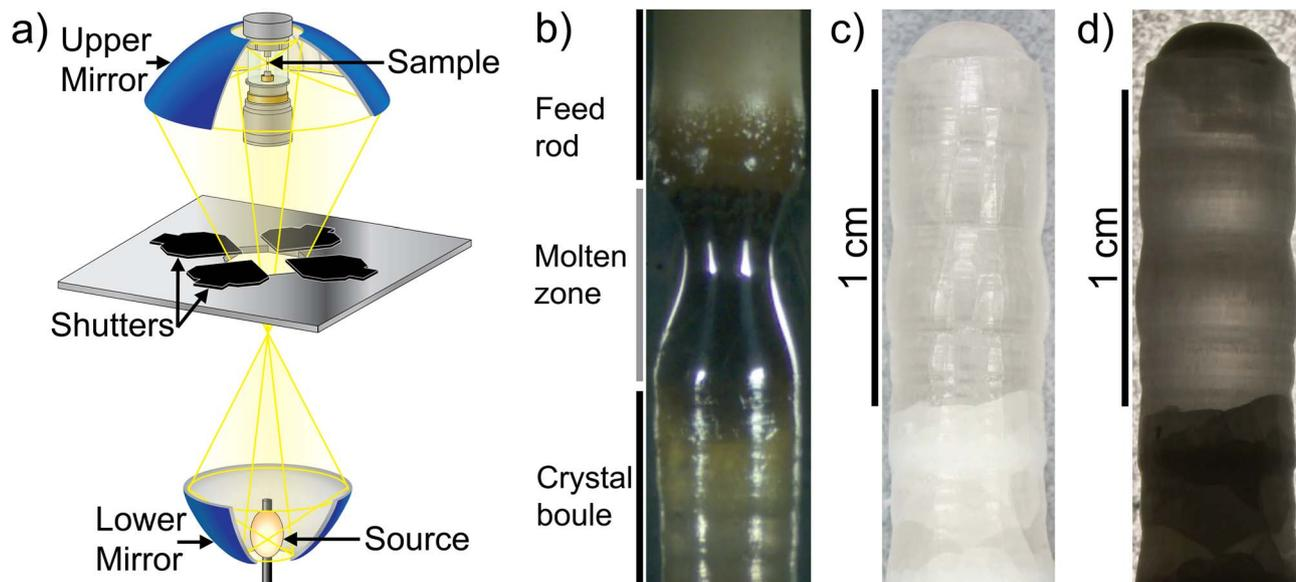
Fig. 1 (a) High-pressure single-lamp floating zone furnace setup. Figure adapted from Scientific Instruments Dresden GmbH.<sup>70</sup> (b) In-progress growth of Li<sub>5.5</sub>-LLNZO rod showing feed rod (top), molten zone (middle), and crystal formation (below). (c and d) Crystal boule segment synthesized with counter-rotation imaged with top lighting (c) and backlighting (d).
