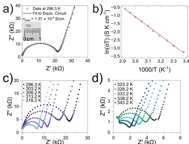
Fig. 7 (a) Nyquist plot of Li<sub>5.5</sub>La<sub>3</sub>Nb<sub>1.5</sub>Zr<sub>0.5</sub>O<sub>12</sub> single-crystal sample from EIS in argon atmosphere at 296.3 K. (Inset) Polished crystal plate for EIS measurements. (b) Arrhenius relationship and line of best fit for  $\ln(\sigma T)$  vs.  $1000/T$  impedance data from 296.3 to 343.2 K ( $R^2 = 0.998$ ). Data shown as black circles, linear fit in red. (c and d) EIS spectra at progressive temperature points from 296.3 to 343.2 K.
