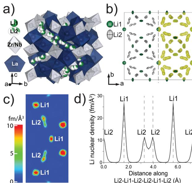
**Fig. 5** (a) Unit cell structure for Li<sub>5.5</sub>-LLNZO determined from neutron single-crystal diffraction. (b) (Left) Anisotropic thermal displacements of Li sites. (Right) Nuclear density iso-surfaces ( $0.399 \text{ fm } \text{Å}^{-3}$ ) based on MEM analysis overlaid on displacement ellipsoids. (c) 2D nuclear density map from MEM analysis through Li1–Li1–Li1 direction. (d) MEM-determined Li nuclear density along Li2–Li1–Li2–Li1–Li2 direction.
