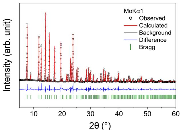
Fig. 3 Rietveld refinement of X-ray powder diffraction pattern for Li<sub>5.5</sub>-LLNZO. The experimental data are shown as black circles, the calculated pattern in red, the difference profile in blue, and calculated Bragg reflection positions in green.
