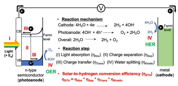
Fig. 1 Schematic illustration of the basic principle of the PEC water splitting system.
