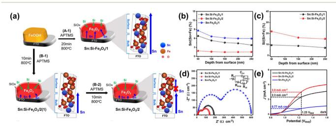
Fig. 12 (a) Fabrication procedures of Sn:Si-Fe<sub>2</sub>O<sub>3</sub>/1 and Sn:Si-Fe<sub>2</sub>O<sub>3</sub>/2. (b) XPS depth profiles of Si and (c) Sn according to the depth from the surface of Sn:Si-Fe<sub>2</sub>O<sub>3</sub>/1–2. (d) EIS measurements at 1.23  $V_{RHE}$ , and (e) J-V curves of Sn:Si-Fe<sub>2</sub>O<sub>3</sub>/1–2, and Sn-Fe<sub>2</sub>O<sub>3</sub>/1. Reproduced from ref. 65 with permission from American Chemical Society, Copyright 2021.
