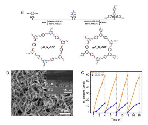
Fig. 6 (a) Rational synthesis of  $g-C_{18}N_3-COF$  and  $g-C_{33}N_3-COF$  by Knoevenagel condensation. (b) The scanning electron microscopy (SEM) micrograph of the  $g-C_{18}N_3-COF$  film from the top view. (c) Photocatalytic  $H_2$  evolution of  $g-C_{18}N_3-COF$  and  $g-C_{33}N_3-COF$  under visible light irradiation by using ascorbic acid as a sacrificial agent. Reproduced with permission from ref. 68. Copyright 2020, American Chemical Society.
