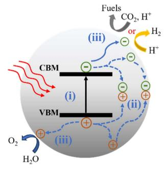
Fig. 3 Scheme of the photocatalytic  $CO_2$  reduction reaction and water splitting for the semiconductor. CBM: conduction-band minimum; VBM: valence-band maximum. (i) Absorption of photons. (ii) Charge separation, migration and recombination. (iii) Surface reactions.
