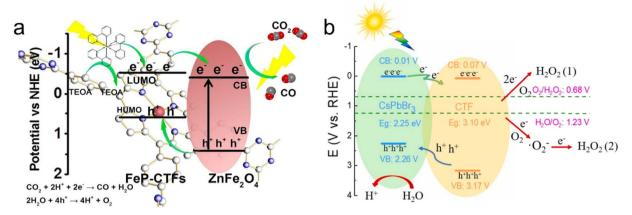
Fig. 16 The proposed charge transfer mechanisms: (a)  $ZnFe_2O_4/FeP-CTF$  for the photocatalytic  $CO_2$  reduction system. Reproduced with permission from ref. 183. Copyright 2021, Elsevier. (b)  $CsPbBr_3/CTF-2$  for photocatalytic  $H_2O_2$  production. Reproduced with permission from ref. 186. Copyright 2022, Elsevier.
