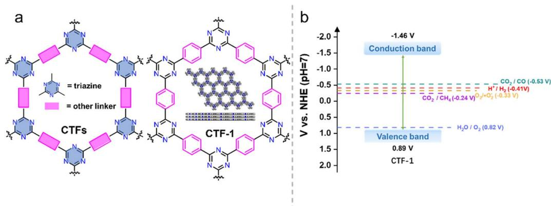
Fig. 1 (a) The structures of CTF and CTF-1. (b) Energy diagram of CTF-1 (ref. <sup>25</sup>) (*t*-BuOK-assisted synthesis).
