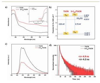
Fig. 2 (a) Diffuse reflectance UV vis spectra of TUCN and  $5-C_{60}/T$  TUCN; inset (Tauc plot), (b) band energy diagram of TUCN and  $5-C_{60}/T$  TUCN, (c) PL spectra of TUCN and  $5-C_{60}/T$  UCN, and (d) TRPL spectra of TUCN and  $5-C_{60}/T$  UCN.
