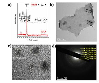
Fig. 1 (a) XRD patterns of TUCN and  $5-C_{60}/TUCN$ , and (b) TEM image, (c) HR-TEM image, and (d) TEM-SAED pattern of 5-C<sub>60</sub>/TUCN.
