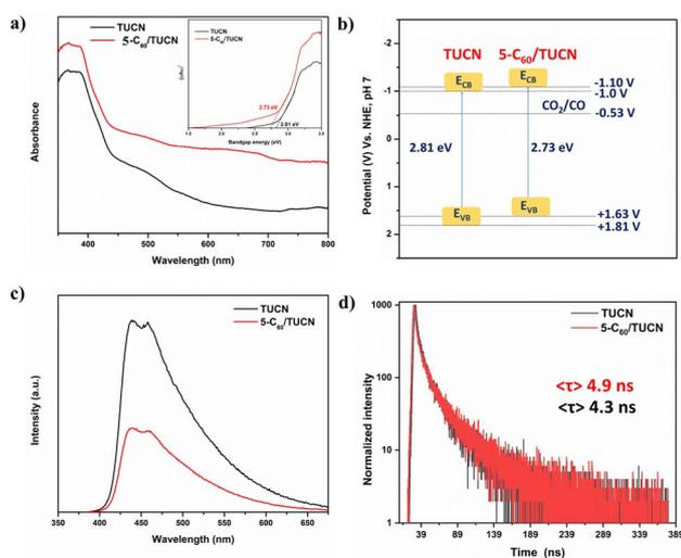
Fig. 2 (a) Diffuse reflectance UV vis spectra of TUCN and 5-C<sub>60</sub>/TUCN; inset (Tauc plot), (b) band energy diagram of TUCN and 5-C<sub>60</sub>/TUCN, (c) PL spectra of TUCN and 5-C<sub>60</sub>/TUCN, and (d) TRPL spectra of TUCN and 5-C<sub>60</sub>/TUCN.
