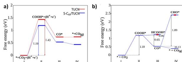
Fig. 3 (a) Calculated free energy diagram corresponding to the reaction path followed by the CO<sub>2</sub> conversion on TUCN and 5-C<sub>60</sub>/TUCN and (b) key steps of CO<sub>2</sub> photoreduction to CO for the 5-C<sub>60</sub>/TUCN system.
