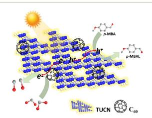
Scheme 2 Plausible mechanistic illustration of dual photoredox CO<sub>2</sub> reduction to CO coupled with p-MBA oxidation over the 5-C<sub>60</sub>/TUCN photocatalyst.
