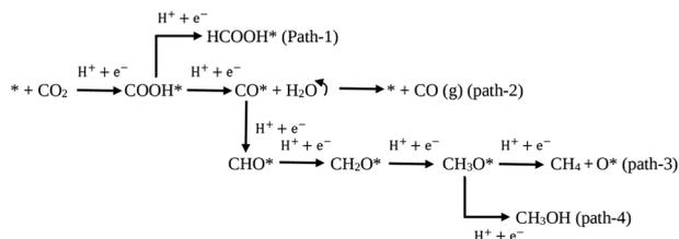
Scheme 1 Proposed reaction paths for CO<sub>2</sub> reduction on the surface of 5-C<sub>60</sub>/TUCN.
