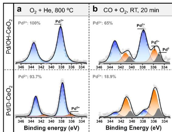
Fig. 3 (a and b) *Quasi in situ* XPS spectra of the Pd 3d core level of Pd/OH-CeO<sub>2</sub> and Pd/D-CeO<sub>2</sub> after (a) as synthesized, and (b) reacting at RT for 20 min.
