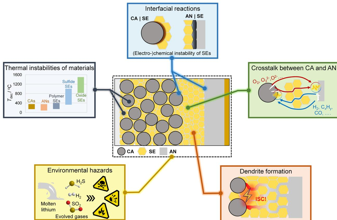
Fig. 3 Safety concerns about SSBs: (I) thermal instability of SSB components; (II) interfacial reactions at CA (cathode)|SE and AN (anode)|SE interfaces; (III) chemical crosstalk between the cathode and anode; (IV) lithium dendrite formation and internal short circuit (ISC); and (V) environmental hazards related to the evolved gases and molten lithium.
