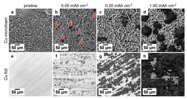
Fig. 3 Pristine (a) Cu micro-foam and (e) Cu foil substrates compared to metallic Li deposited on (b-d) Cu micro-foams and (f-h) Cu foil. Using a current density of  $0.1 \, \text{mA cm}^{-2}$ , Li amounts equal to (b and f)  $0.05 \, \text{mA}$  h cm<sup>-2</sup>, (c and g)  $0.20 \, \text{mA}$  h cm<sup>-2</sup>, and (d and h)  $1.00 \, \text{mA}$  h cm<sup>-2</sup> were deposited. Arrows in (b) mark deposited Li structures.
