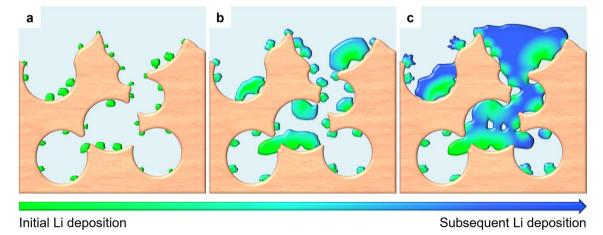
Fig. 5 Schematic representation of the continuous growth of Li structures inside the Cu micro-foam pores during Li electrodeposition at a current density of 0.1 mA cm<sup>-2</sup>. A continuous color scheme denotes the progressing expansion of the Li structures from (a) initial (green) to (b and c) subsequent (blue) electrodeposits.
