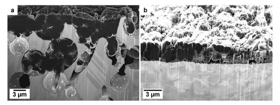
Fig. 4 Cryo-FIB cross-section SEM images of (a) Cu micro-foam and (b) flat Cu foil after electrodeposition of an amount of metallic Li equal to 0.20 mA h cm<sup>-2</sup> using a current density of 0.1 mA cm<sup>-2</sup>
