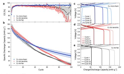
Fig. 7 (a) Coulombic efficiency and (b) average discharge capacity measured when charge/discharge cycling NCA||Cu micro-foam (blue), NCA||Cu foil dendritic (red), and NCA||Cu foil flat (black) cells with a current density of 0.2 mA cm $^{-2}$  (0.2C) for 100 cycles at 40 °C. The results of three equivalent cells are averaged for every set-up. Corresponding charge/discharge voltage profiles for cells with (c) Cu micro-foam, (d) dendritic Cu foil, and (e) flat Cu foil negative electrodes.
