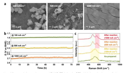
Fig. 4 Monitoring the stability, morphology and structure of FeNiCr/FF during the OER with independently controlled current density from 100 mA cm $^{-2}$  to 1000 mA cm $^{-2}$ . (a) SEM images, (b) chronopotentiometry profiles, and (c) Raman spectra.
