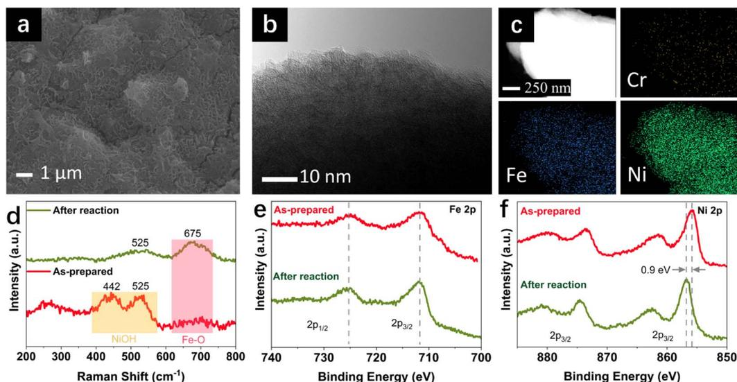
Fig. 3 Characterization of FeNiCr/FF after a three-day OER stability test at  $500 \text{ mA cm}^{-2}$ ,  $50^\circ \text{C}$ , and  $5 \text{ M KOH}$ : (a) SEM, (b) HRTEM, (c) EDS mapping, (d) Raman spectra, and high-resolution XPS spectra for (e) Fe 2p and (f) Ni 2p.
