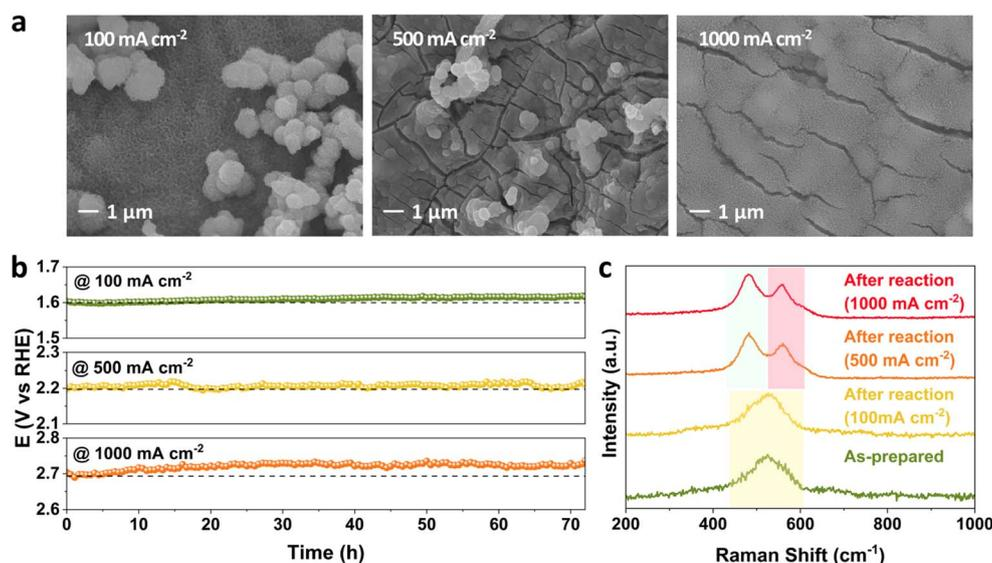
Fig. 4 Monitoring the stability, morphology and structure of FeNiCr/FF during the OER with independently controlled current density from  $100\text{ mA cm}^{-2}$  to  $1000\text{ mA cm}^{-2}$ . (a) SEM images, (b) chronopotentiometry profiles, and (c) Raman spectra.
