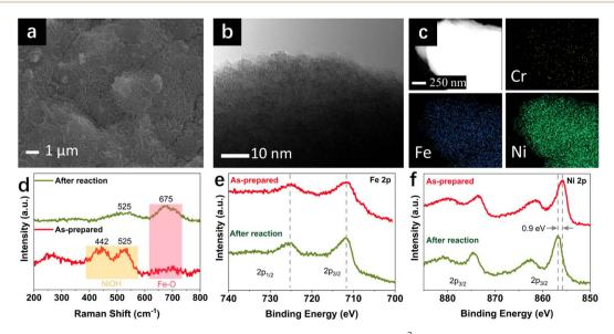
Fig. 3 Characterization of FeNiCr/FF after a three-day OER stability test at 500 mA cm<sup>-2</sup>, 50 °C, and 5 M KOH: (a) SEM, (b) HRTEM, (c) EDS mapping, (d) Raman spectra, and high-resolution XPS spectra for (e) Fe 2p and (f) Ni 2p.
